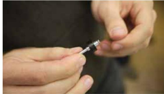
Run the Dremmel on high speed and create a groove with a sharp object
