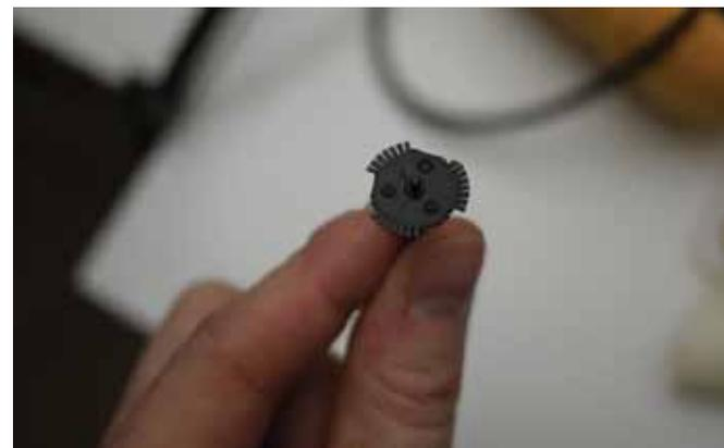
Tape the teeth so the disc has three teeth in total in the end
